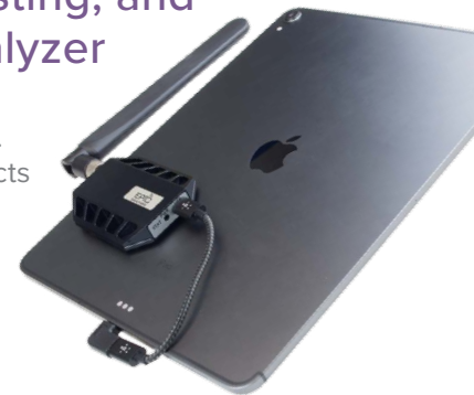
PRISM, shown mounted to a tablet, weighs under 24 grams (6 oz.)
