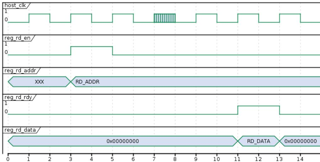
Fig. 2.5: Register Read Interface Timing Diagram (VAR\_LATENCY\_REG\_RD=1)
