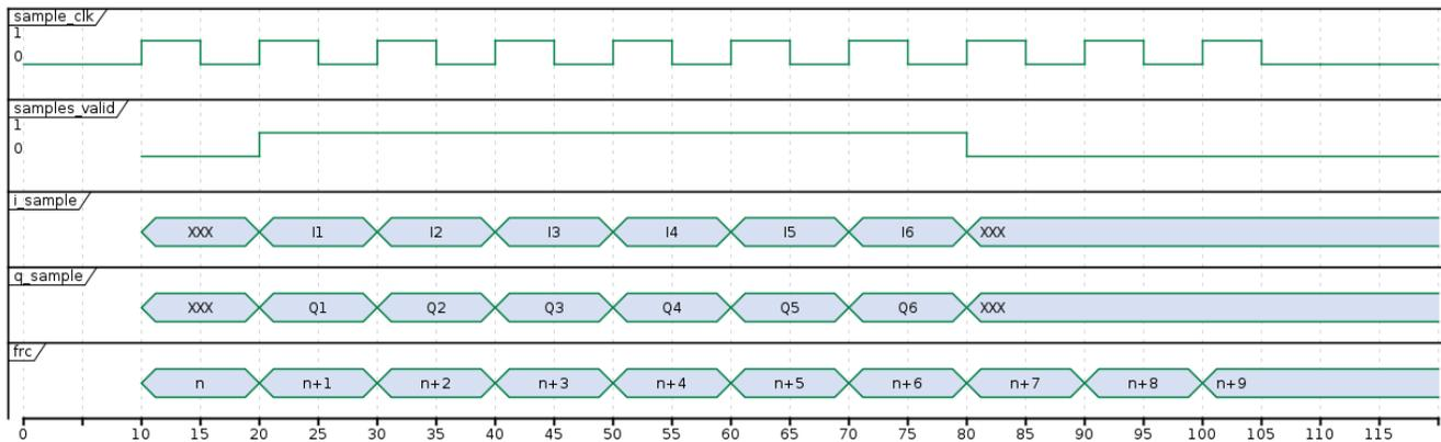
Fig. 2.6: Rx Data Interface Timing Diagram
