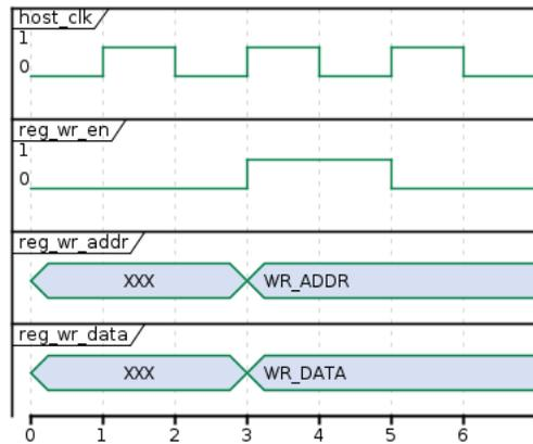
Fig. 2.3: Register Write Interface Timing Diagram
