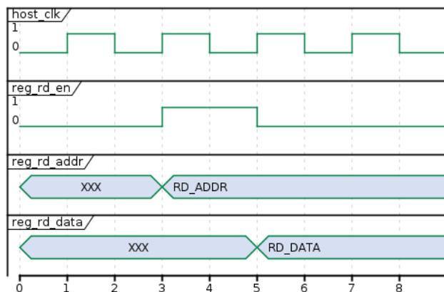
Fig. 2.4: Register Read Interface Timing Diagram (VAR\_LATENCY\_REG\_RD=0)
