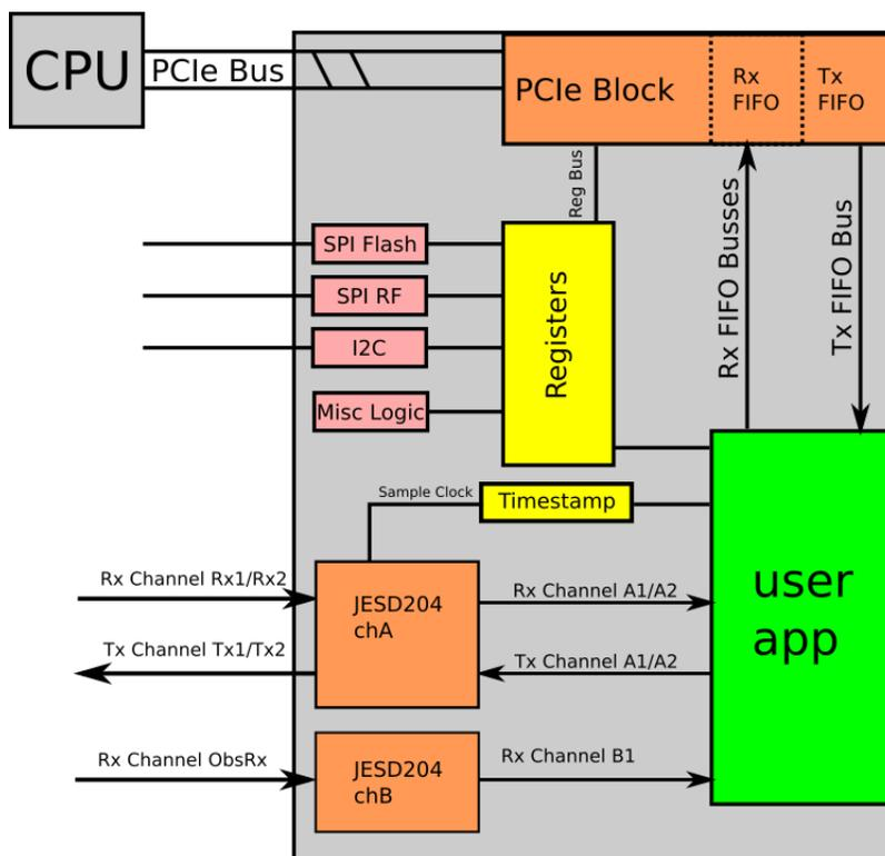
Fig. 2.1: Sidekiq X2/X4 Simplified Block Diagram
