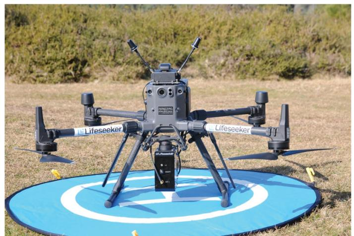
Figure 2: Lifeseeker UAS with sensor pod attached
