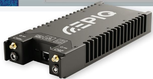
**Figure 4:** New Epiq X40 software defined radio (SDR) with embedded GPU, now shipped with an evaluation copy of OmniSig.
