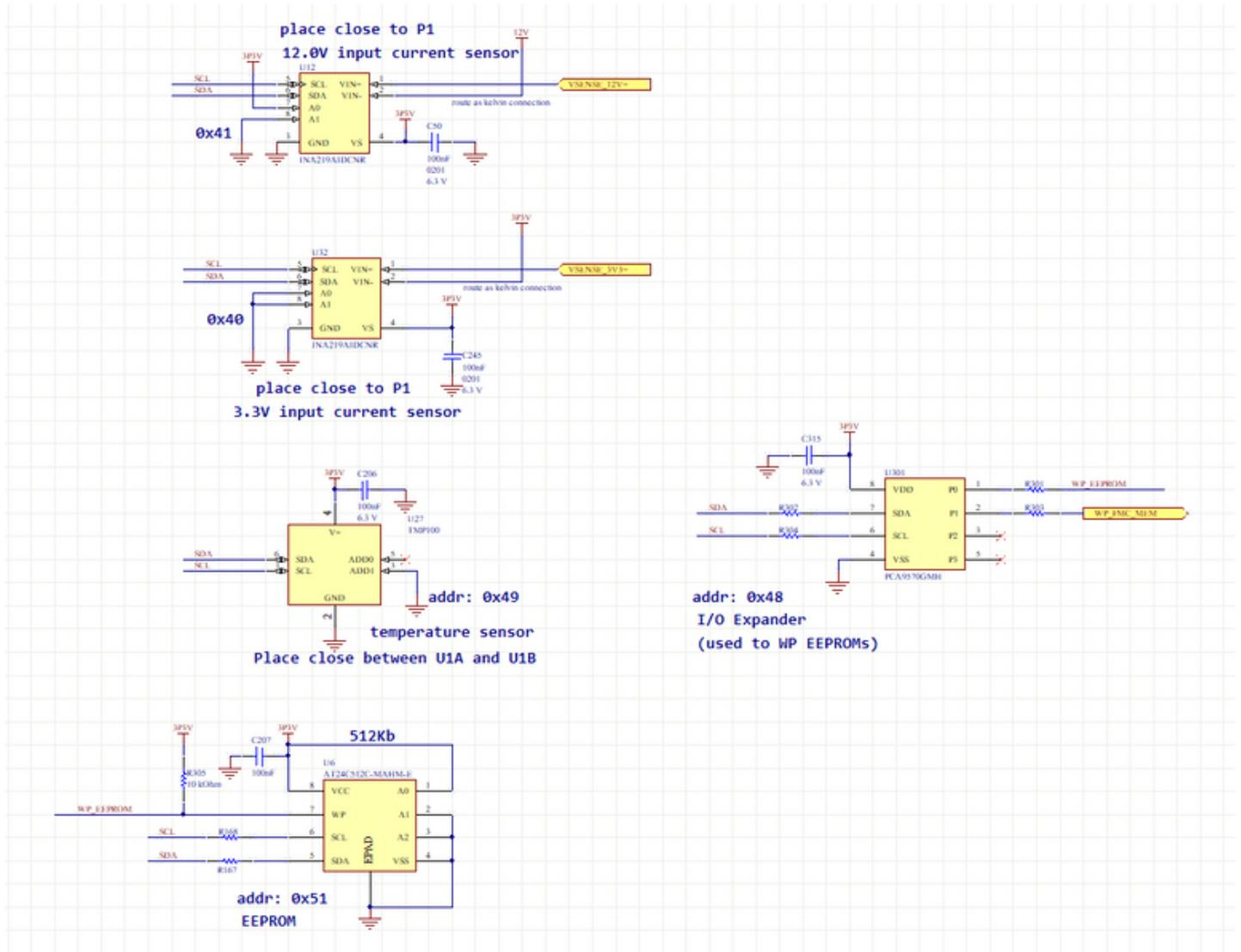
Figure 6: Sidekiq X4 I2C devices
