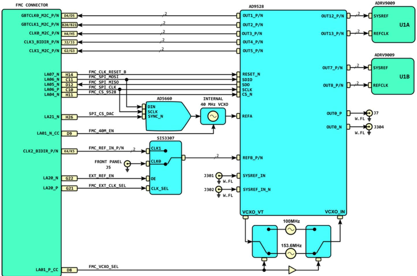
Figure 7: Sideiq X4 rev B JESD Clocking Structure
