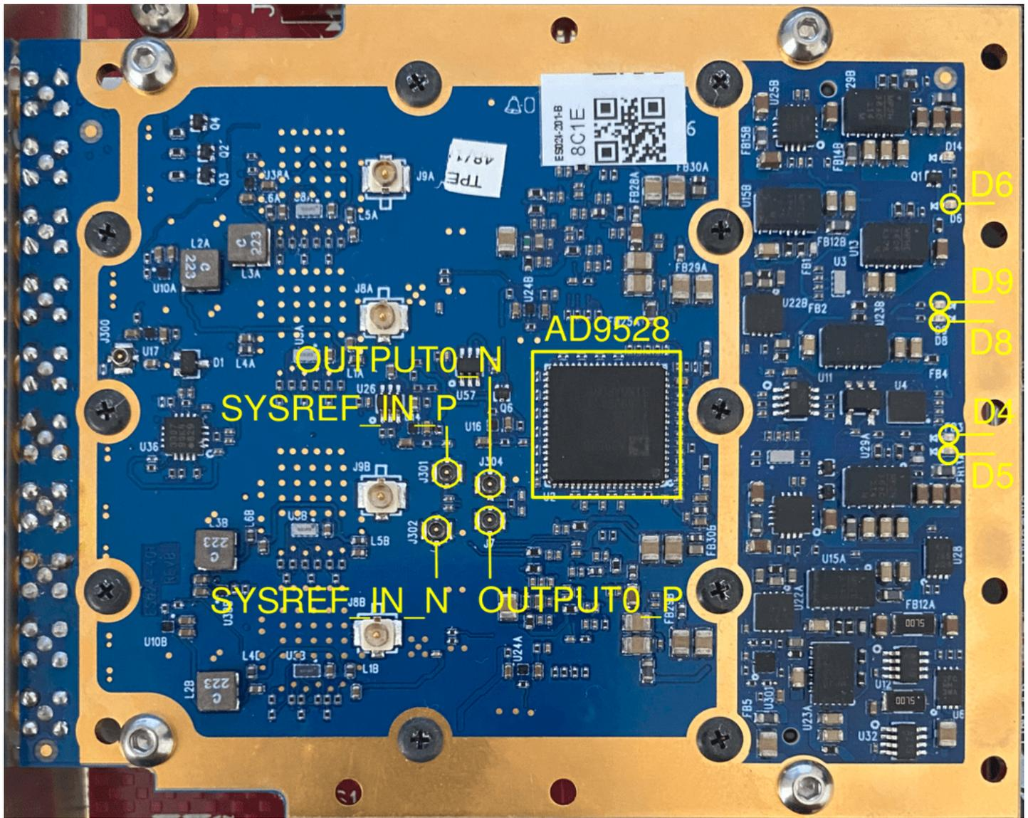
Figure 3: AD9528 clock IC locations
