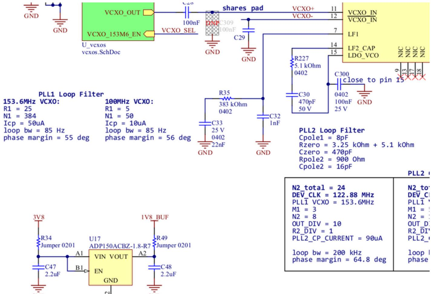
Figure 2: AD9528 default configurations
