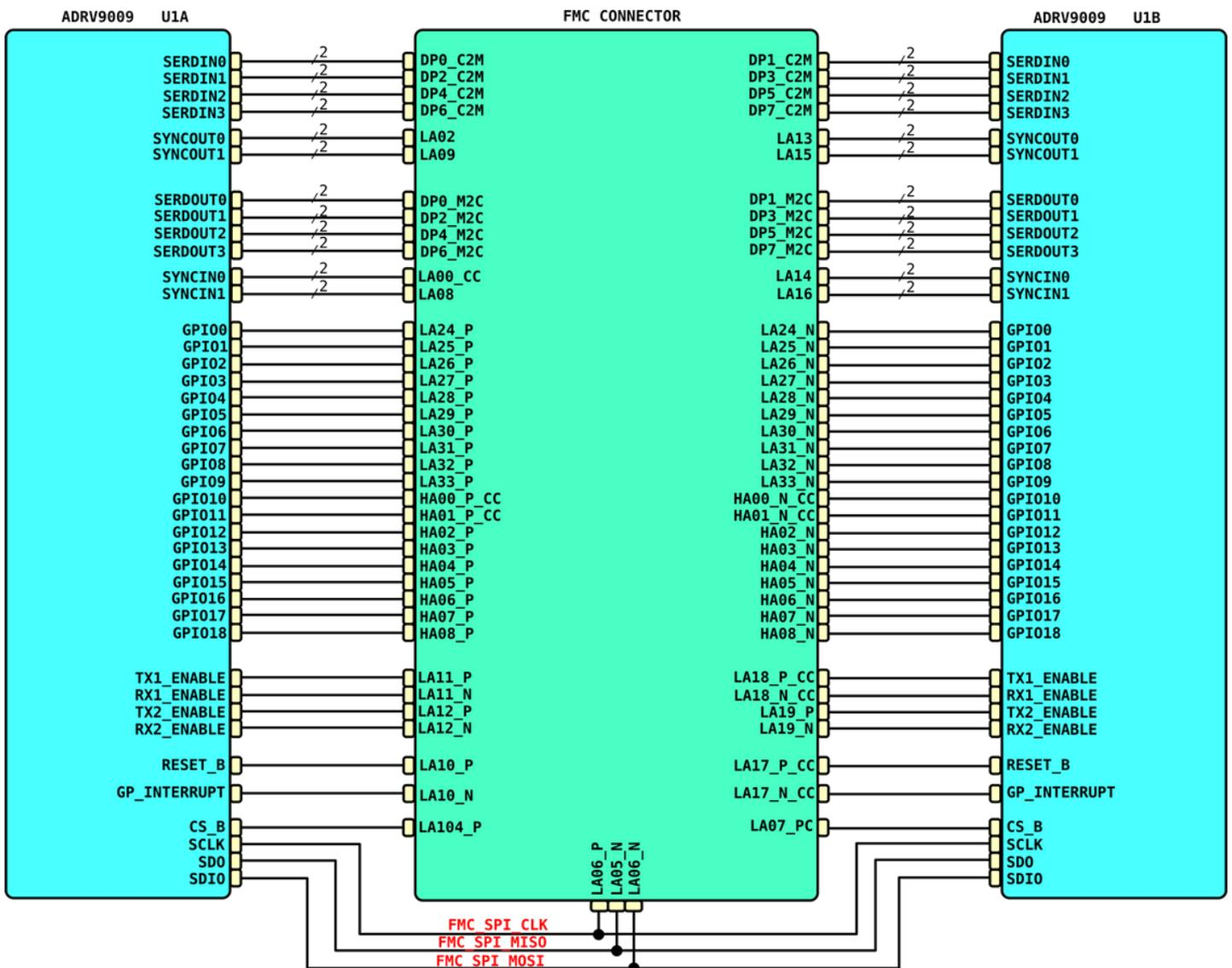
Figure 4: FMC connections to ADRV9009 RFICs
