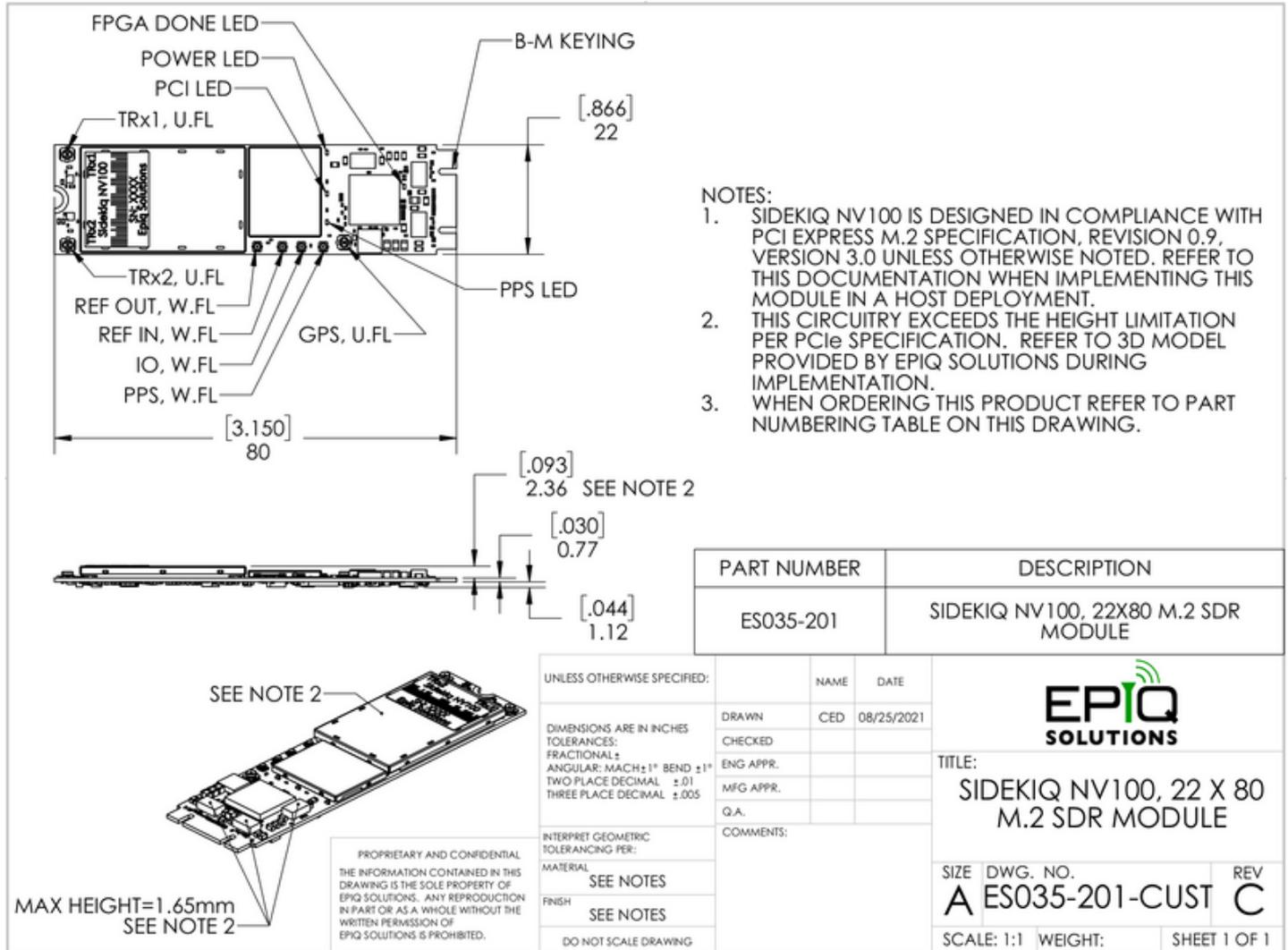
Figure 11: Sidekiq NV100 dimensioned drawing
