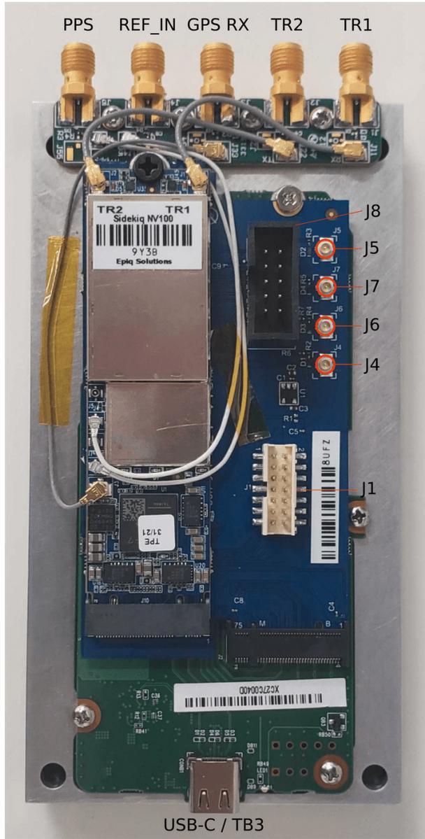
Figure 8: Sidekiq NV100 JTAG Fixture
