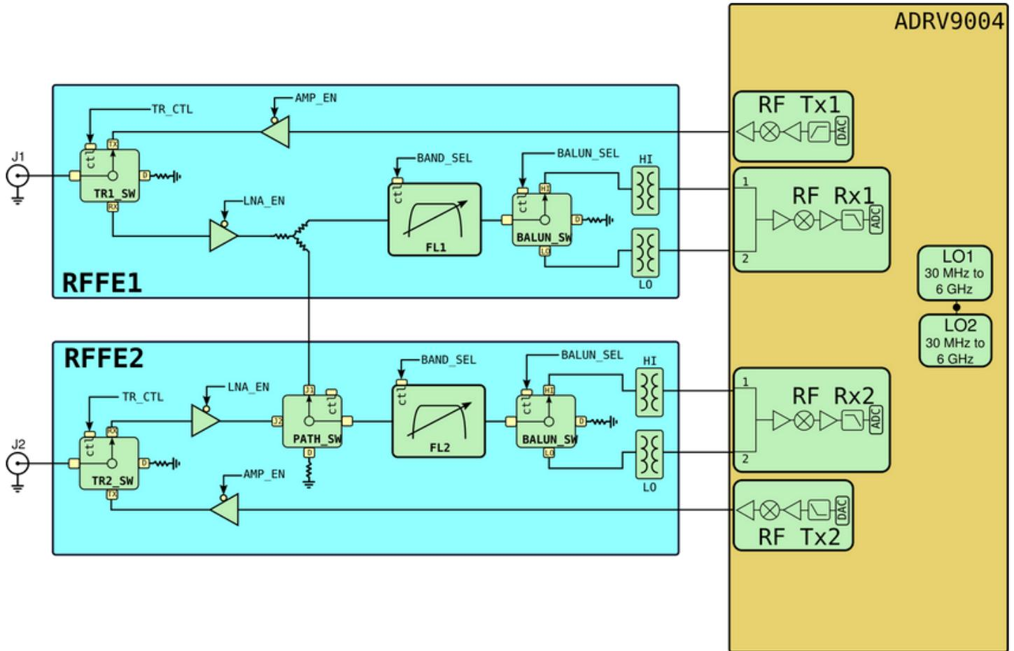
Figure 12: Sidekiq NV100 RF Front End Block Diagram
