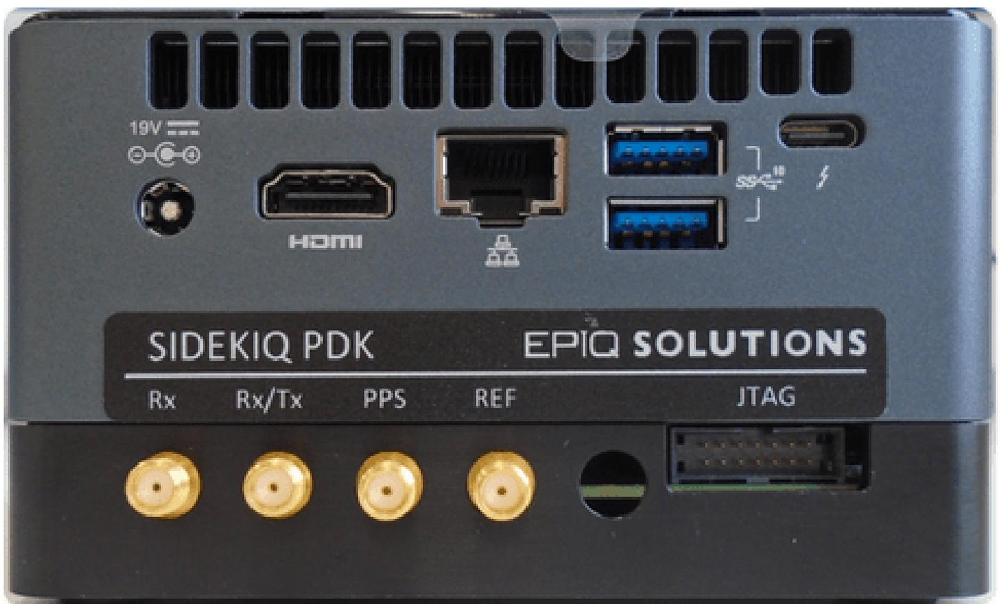
*Figure 6: Sidekiq NUC hardware I/O interfaces*
