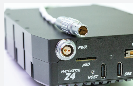
View of mating power connectors
