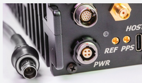
View of mating power connectors
